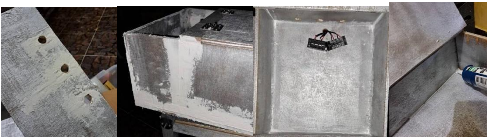
Figure 11: Wood Filling and silicon on the Body Structure
